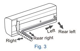
(2) When selecting to lead out the pipe from the left or right, please cut the corresponding hole in the bottom case. (As shown in Fig. 4)
