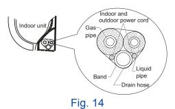
(2) Reserve a certain length of drain hose and power cord for installation when binding them. When binding to a certain degree, separate the indoor power and then separate the drain hose. (As shown in Fig. 15)
