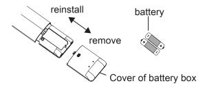
1. Press the back side of remote controller marked with €, as shown in the fig, and then push out the cover of battery box along the arrow direction.
