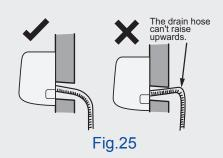
Slant the drain hose slightly downwards. The drain hose cant be curved, raised and fluctuant, etc.(As shown in Fig.26)
