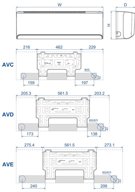
NOTE: Choose the diameter of piping hole according to the pipe-holesleeve.
