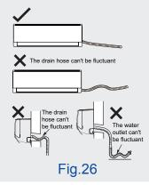
The water outlet cant be placed in water in order to drain smoothly.
