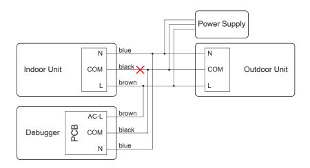
The power cord of the debugger can be connected to the terminal board of the IDU or the ODU. Note that the communication wire(black wire) of the IDU main board must be disconnected from the terminal board. As shown below:
