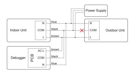
The power cord of the debugger can be connected to the terminal board of the IDU or the ODU. Note that the communication wire (black wire) of the ODU must be disconnected from the terminal board. As shown below:
