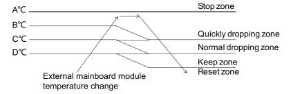
Mainboard module overheating protection temperature:
