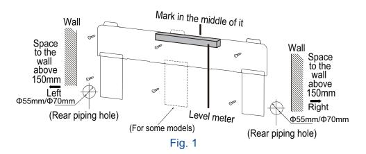
(2) When installation is finished, pull the mounting plate by hand to confirm whether it is fixed tightly. The force distribution among all screws should be uniform.
